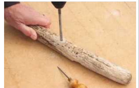
▲ Pic.3 A bradawl is handy to start each hole. Drill right through every branch with a flat or dowel bit
